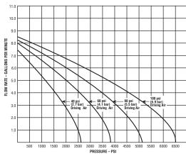
**S-218-GJC-()**—This 10.5 hp, double-acting piston pump services oil, water and compatible chemicals. It is ideal for hydrostatic testing, machine operations, charging accumulators and for deep-hole applications.
