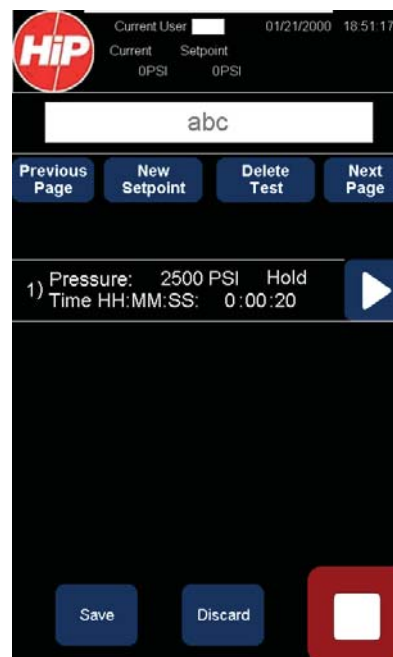
FIG. 15 Test Setpoint Overview Screen
