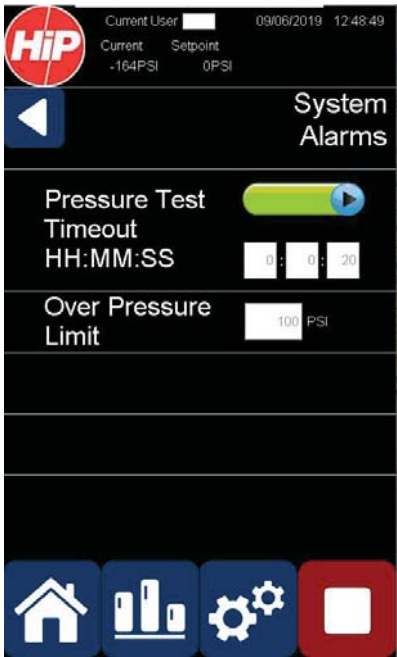
FIG. 23 System Alarms Screen
